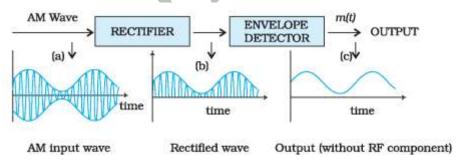
Block diagram of a detector for AM signal. The quantity on y-axis can be current or voltage.
