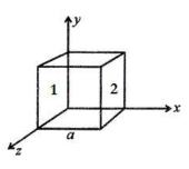
**SOL:** Surface (1) E = 0 at x = 0,  $\phi = 0$  flux entering to the cube is zero. Surface (2) flux entering to the cube =  $2 a \times a^2 = 2 a^3$
