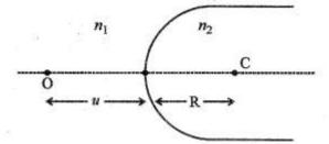
(b) When the image formed above acts as a virtual object for a concave spherical surface saparating the medium  $n_2$  from  $n_1$  ( $n_2 > n_1$ ), draw this ray diagram and write-the similar (similar to (a)) relation. Hence obtain the expression for the lens maker's formula.
