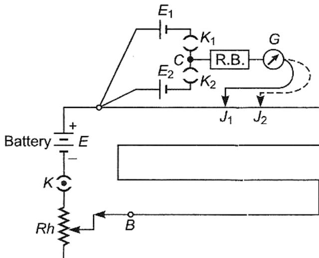
The main circuit comprises of battery of emf  $E$ , key ( $K$ ) and rheostat ( $Rh$ ). The auxiliary circuit comprises of two primary cells of emfs  $E_1$  and  $E_2$ , galvanometer, jockey and resistance Box ( $RB$ ) to prevent large current flowing through the galvanometer.
